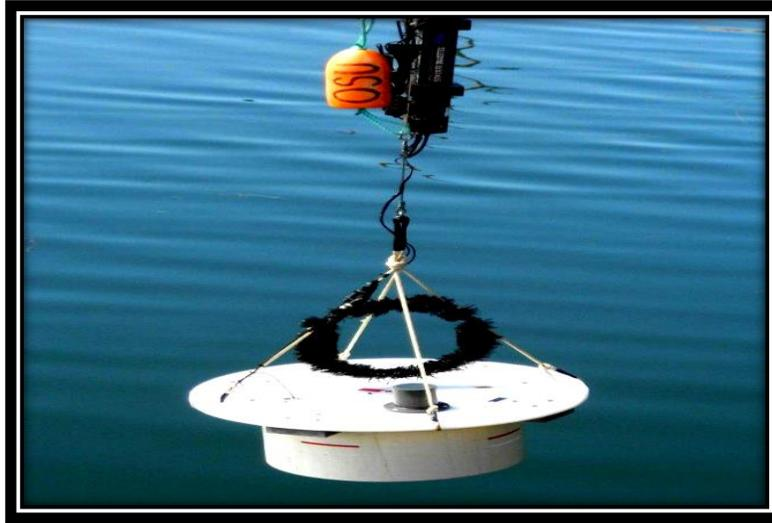
BMFC. Power from the BMFC maintains the modem and a chemical sensor (optode) interfaced with the modem.
